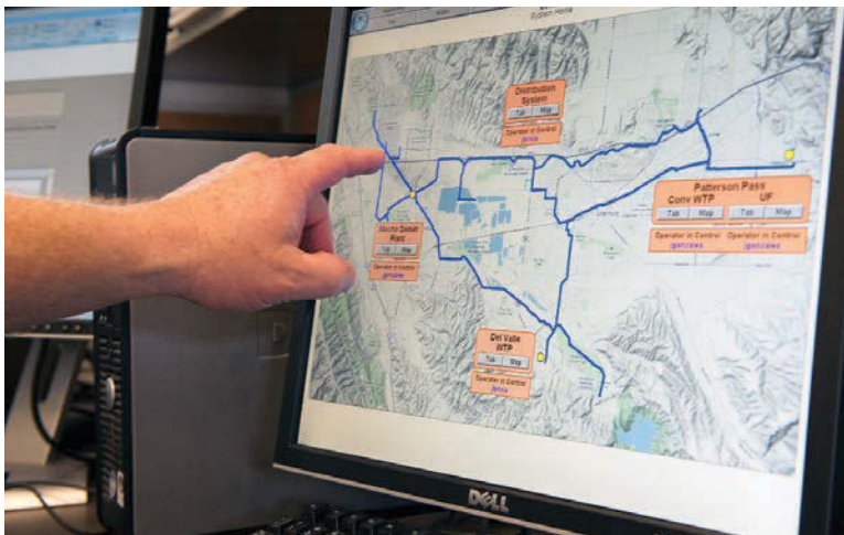
The SCADA system enables the plant to be permitted as an unstaffed facility (Invensys Wonderware software; system integrator Wunderlich-Malec).
