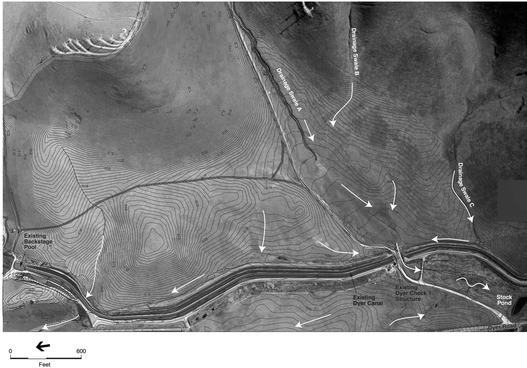
Figure 3.2-2 Existing Drainage Gradients, Dyer Reservoir
