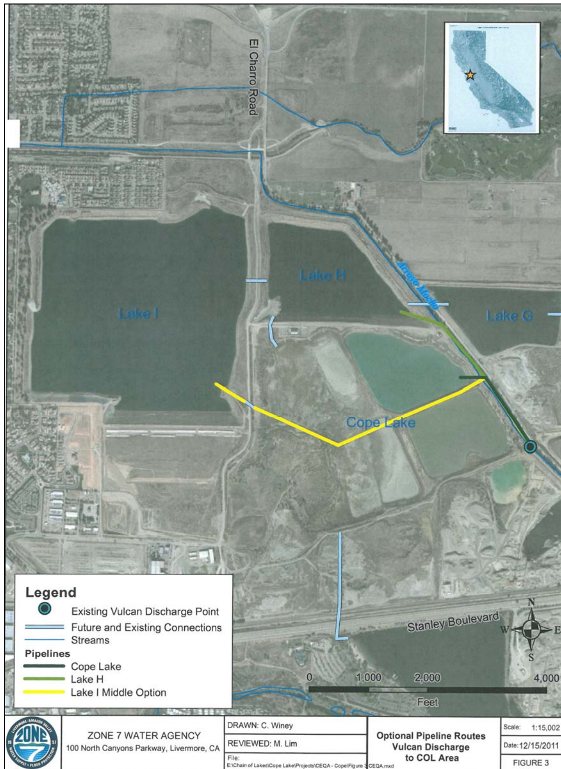
Figure 3. Vulcan Discharge Pipeline – Proposed Pipeline Routes
